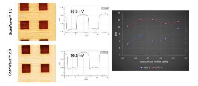
Signal to Noise comparison for ScanWave™ 1.5 vs ScanWave™ 2.0 on a standard Al-dot sample
