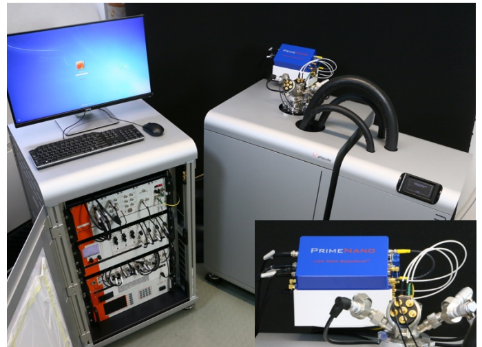
LT ScanWave™ sMIM system with Electronics control rack, closed cycle cryostat, 9T magnet and Low Temp sMIM electronics.
